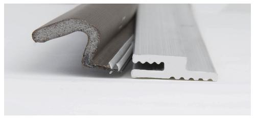
Aluminum retainer is 5 to 7 times thicker than others preventing damage from heavy use. Oversize foam seals flex to accommodate warps, dents and twists in any door. The unit can be adjusted to doors that are up to 1" away from door stop. Foam seals can be removed to paint doors. (Requires special knowledge.) Mitering or notching is not required.
